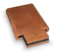
IN electrodes are made from high-purity copper of grades E, SE or OF-CU. Casting blocks are hot extruded and the precise copper profile is produced through subsequent drawing.
